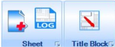
The **Paper space** tab contains options to place the created drawings in a paper space sheet and edit them. Sheets are predefined in the Viskar BIM. The user can also create new sheet for the project requirements. Title block can be designed and edited according to the requirement.
